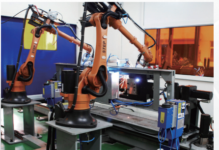
Enforce Beam (Elevator) Welding
