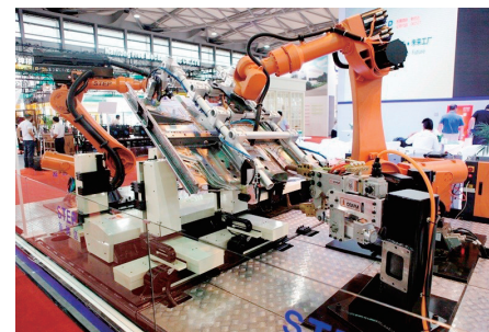
Car Frame Flexible Spot Welding
