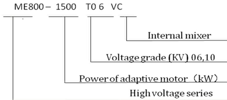
Fig.1-1 Description of inverter model
