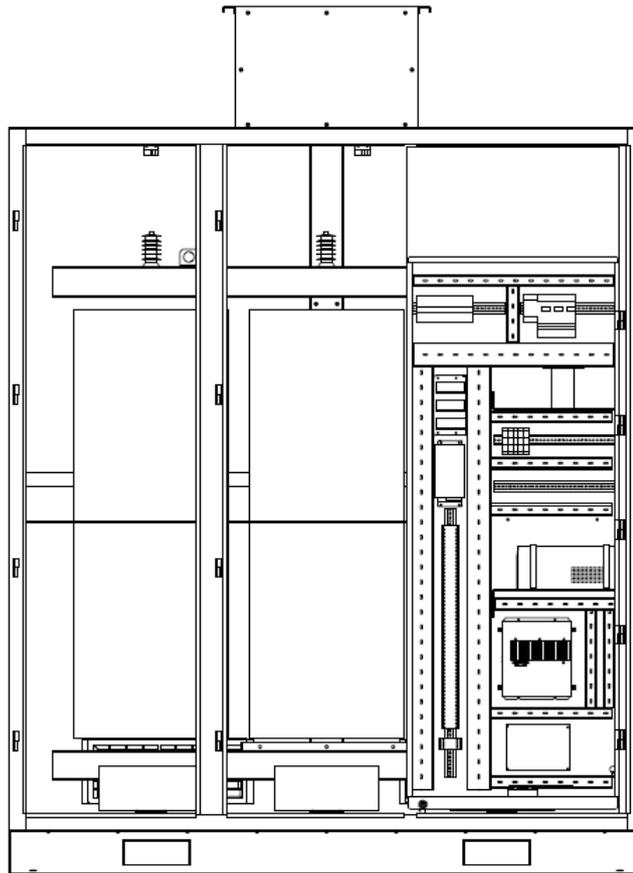
Fig.2-6 Inside of transformer cabinet
