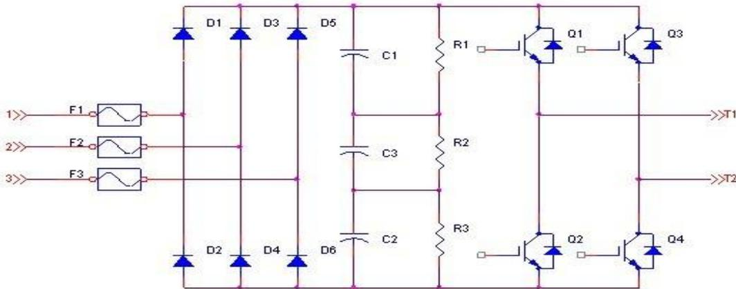
Fig.2-9 Power unit topological diagram
