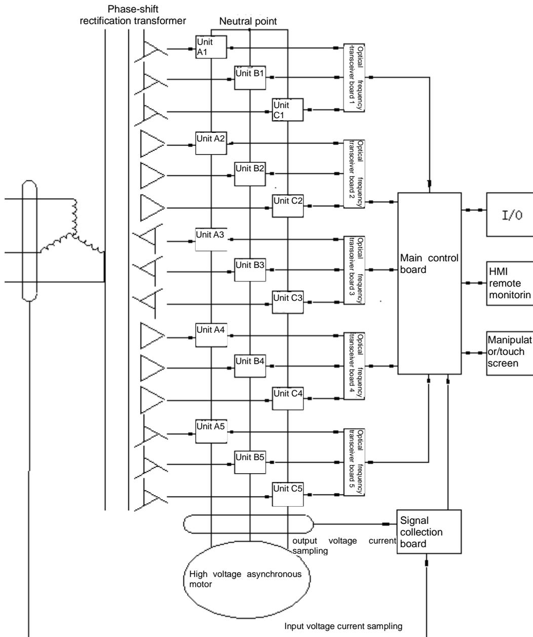
Fig.2-8 Principle diagram of high voltage inverter system(6kV as an example)
