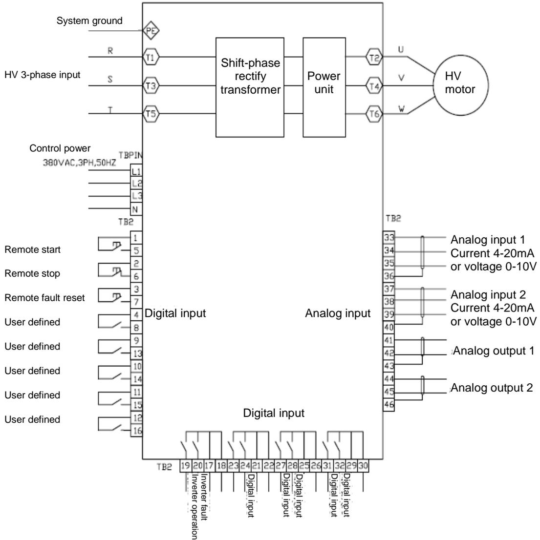
Fig.3-3 Typical system external interface diagram
