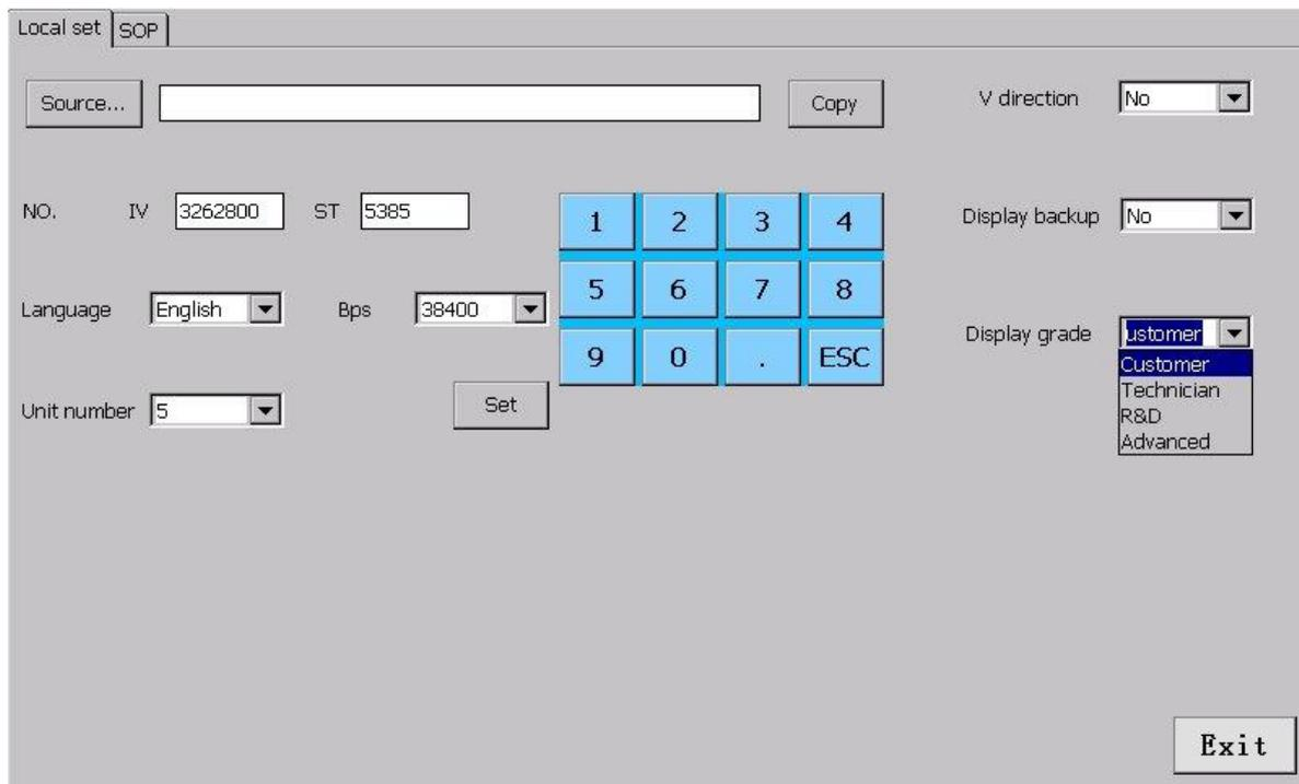
Fig.4-16 Local setting interface of touch screen
