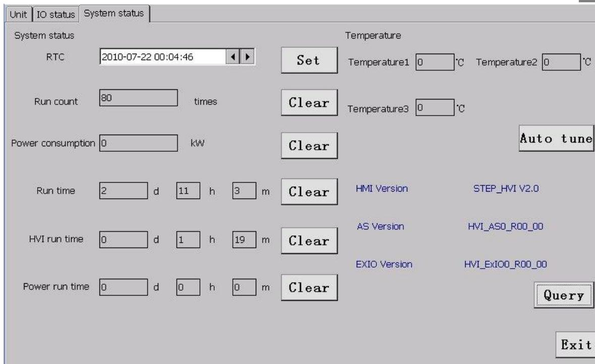
Fig.4-7 System status interface of touch screen
