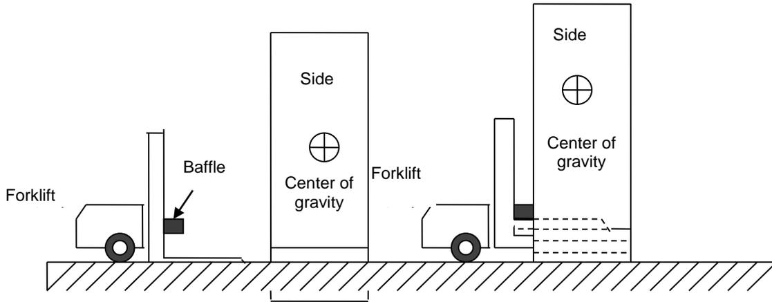
Fig.3-2 Correct way to use the forklift
