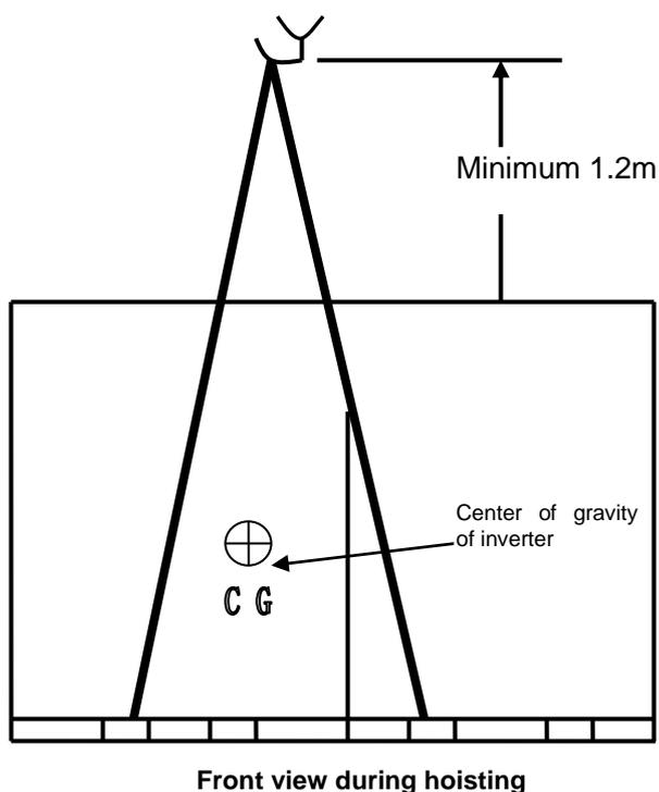
**Fig.3-1 Center of gravity of inverter must be noted when steel wire is used for hoisting**
