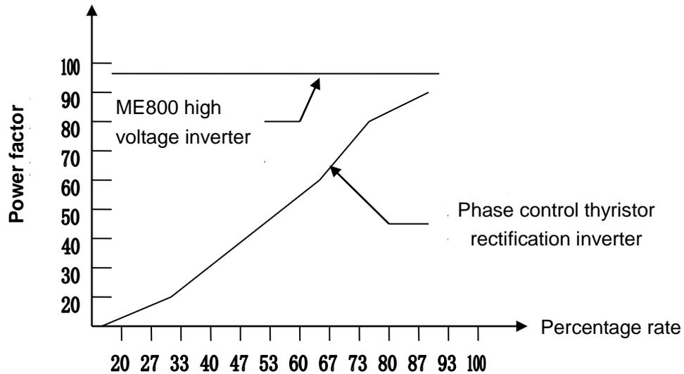
Fig.2-4 Power factor comparison between ME800 high voltage inverter and phase control thyristor
