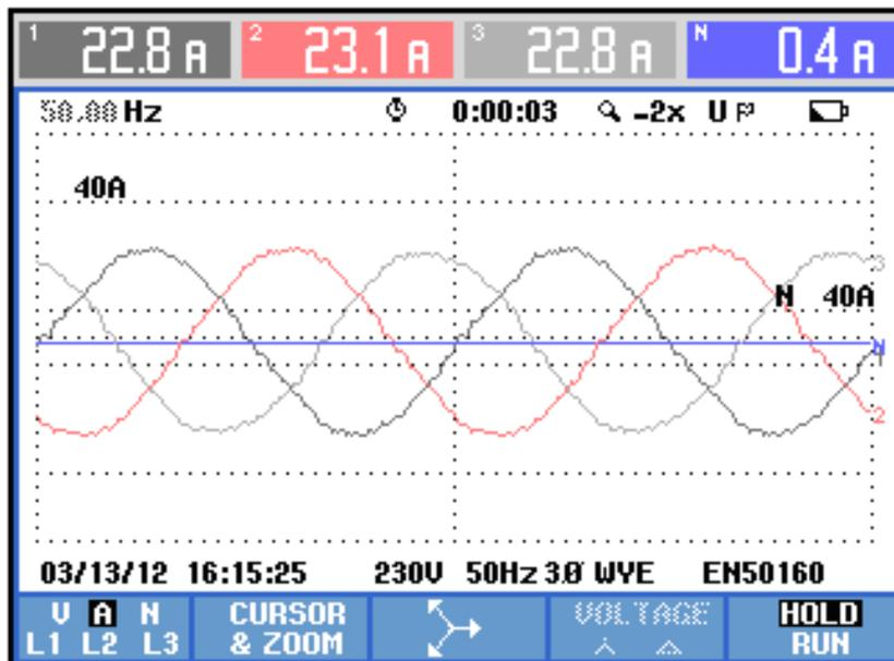
Fig.2-1 Input 3-phase current wave form
