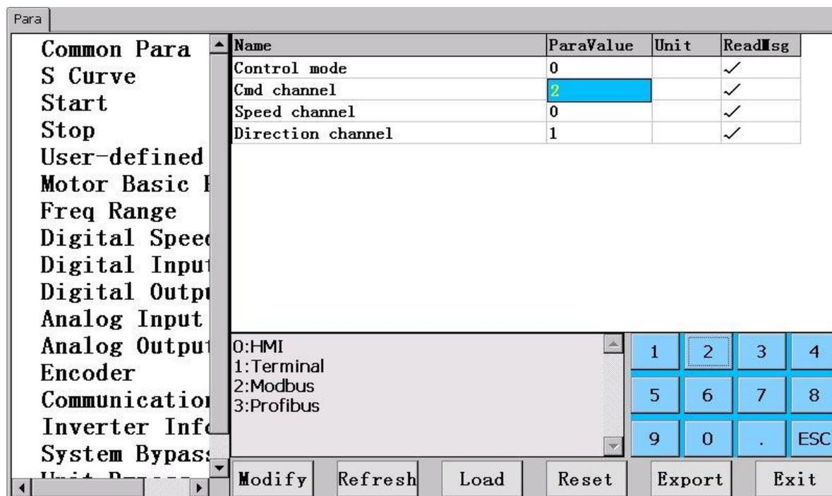
Fig.4-14 Parameter setting interface of touch screen
