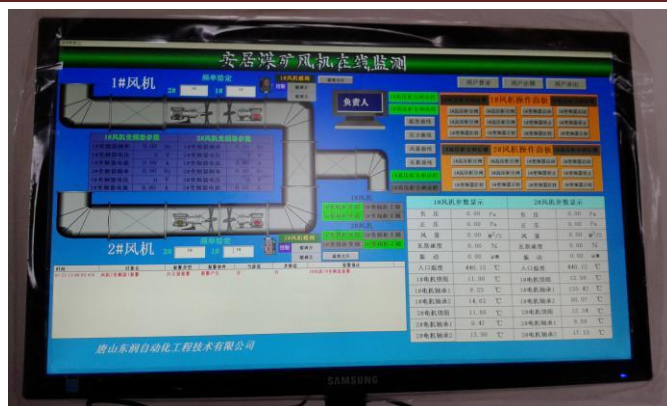
FIG. 4 Counter-rotating fan PLC control interface
